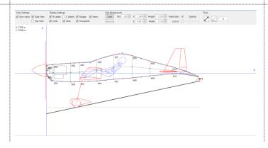
The LCL line editor can also display: other geometric elements of the aircraft, a number of internal components such as occupants and the engine, as well as the ground position—both in-flight and on-ground.
