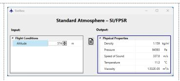
• Lists the characteristics of the standard atmosphere at a given altitude
