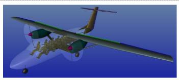
For passenger transport aircraft, the seat layout can be quickly determined by specifying the row spacing and the number of seats per row.
