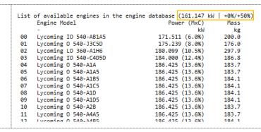
Generates a list of engine candidates to power the aircraft based on the computed power requirement (Design Level 1).
